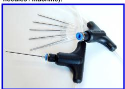
The fluid supply to each needle is controlled by self-compensating, flow-regulating valves; these valves are tamper-proof (encased in the T-piece immediately above the needle), require no user adjustment, and are pre-set to deliver 35 ml/min (+/- 10%) from each needle.
