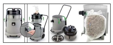
If the vacuum bag requires replacement this should be undertaken by a competent person utilising original Numatic parts, PPE, and containment measures appropriate to the dust hazard to prevent exposure to, and spread of, dust when changing the bag; do not attempt to change the bag unless you can satisfy this requirement. Bag change process: disconnect the vacuum hose, fit the dust cap, switch off the vacuum, un-clip the lower
