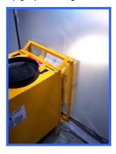
Once in place lock the castors to stop the DFU from moving, connect the machine to a power supply, switch on <u>and then</u> immediately remove the circular transit cover from the machine inlet.
