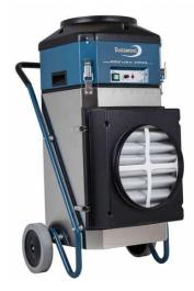
Technical Date: 110v single phase electric motor, power 500W, connection via trailing lead with 110v 16A plug. Airflow variable control 0–1850 m3/hr. Dimensions 970 x 600 x 340mm, weight 25kg, sound level 62 – 74 dB(A), inlet and discharge spigot 315m diameter. Max. negative pressure 500Pa, ultimate filter: Microfilter H13 HEPA 99.995%.
